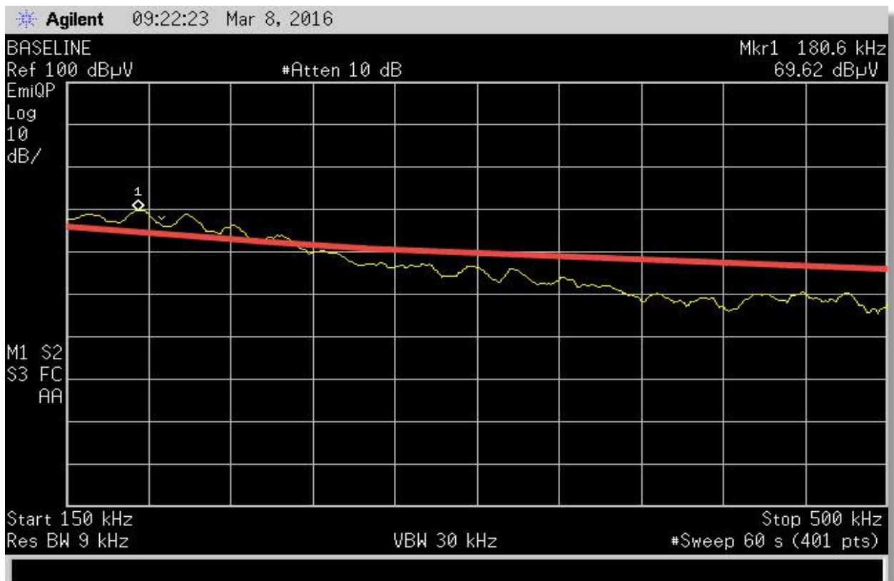
No Filter Installed, Quasi-Peak Plot
